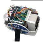
The OT200 Compact Ceiling Hoist is designed to be 'easy to maintain' ensuring that upon a service or inspection, all but the wheels can be serviced on the rail. This removes the need to dismantle the tracking system on every call out.
