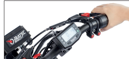
180 mm disc, two mechanical brakes, two aluminium levers with parking brake.
