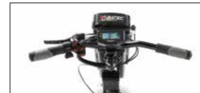
Monolever brake and accelerator handlebar for hemiplegics.
