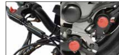
140 mm disc, two mechanical brakes, two aluminium levers with parking brake.
