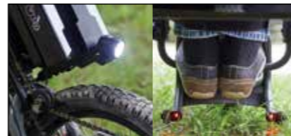
700 lumens front light. Double LED taillight on the stand.
