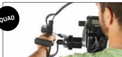
BATEC SHIFT LEVER. Shimano REVO 8 gear shifter.
