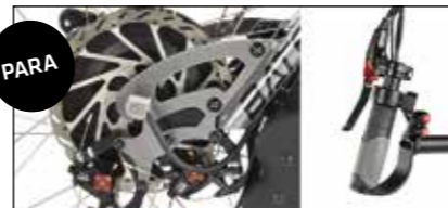
Double sensor clamp with Saccon current cut-off levers and 200/203 mm rotor disc double parking brake.
