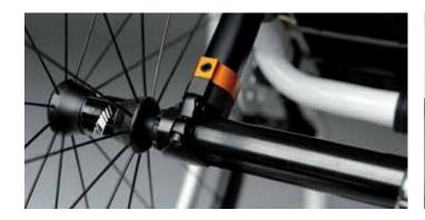
Rigid axle assembly with height adjustment. Oval shapes, forged parts, wider clamps and 'cathodic coating' ensure extreme rigidity, silence and allows +/-1 cm fine tuning of rear seat height.
