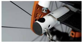
Lightweight back angle adjustment. Helium offers fixed, folding and folding/double locking backrests. Easy to adjust from -15 to +31 degrees to the frame. Less materials, less weight.
