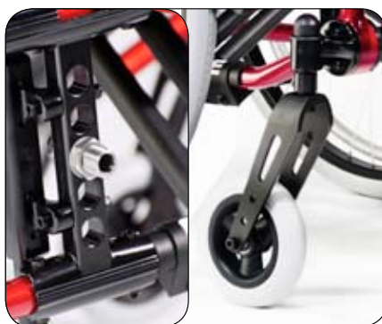
Seat height and camber adjustment via rear axle plate, castor housing and fork (standard feature)
