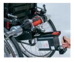
The LIGHT DRIVE is controlled with a joystick and yet remains as manoeuvrable and easy to use as a manual chair. By releasing the clutch you can free wheel giving you the choice when to use it. The compact design means it fits into the smallest of cars or the luggage compartment on the plane.
