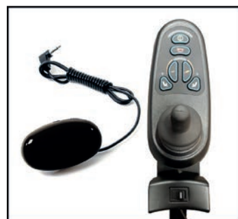
VR2 drive control with LED marker switch & Buddy button for 10" seat lift
