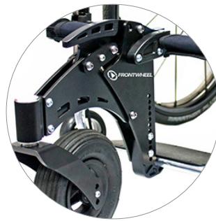
Robust three point connection to frame
